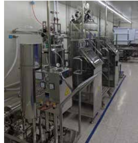
Equipment image from near to far: magnetic tank → configuration tank #3 → configuration tank #2 Implementation period: January 2020 to December 2020 Source: Pegavision
